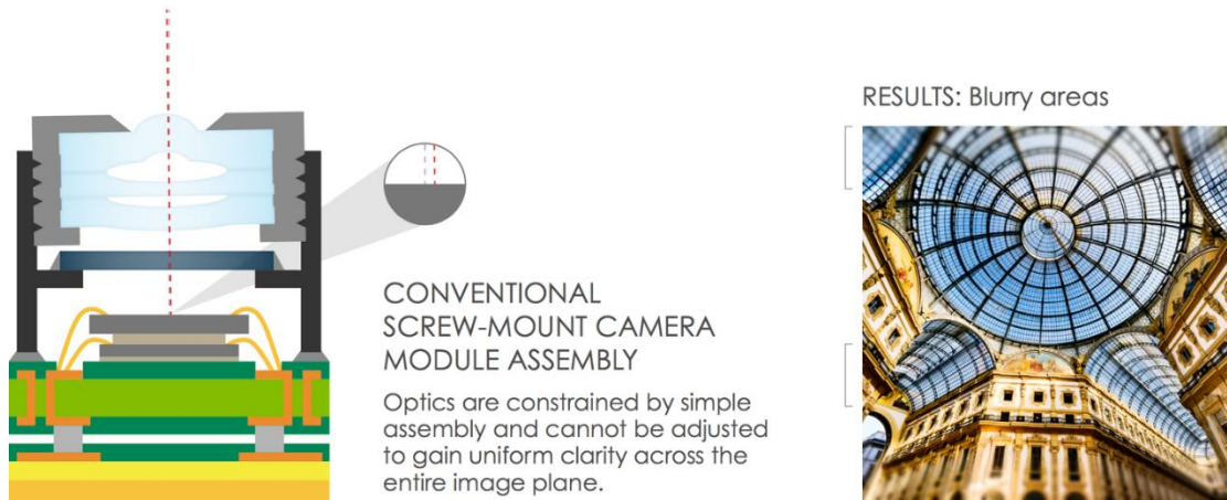
FIGURE 1: CONVENTIONAL LENS & SENSOR ASSEMBLY
