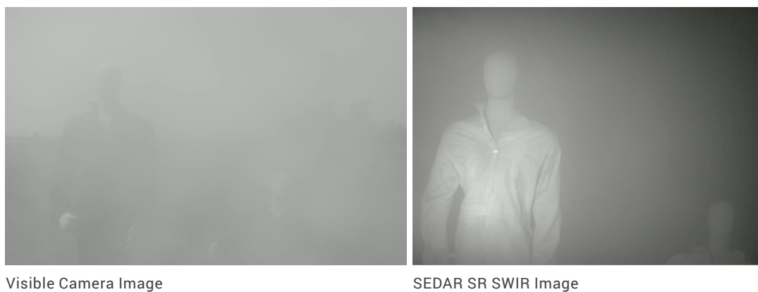
FIGURE 15: SEDAR SR OPERATION IN DUSTY OUTDOOR ENVIRONMENT AT 10 METERS
