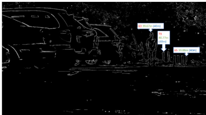
FIGURE 11: OBJECTS @ 40 METERS IN HIGH AMBIENT LIGHT ENVIRONMENT
