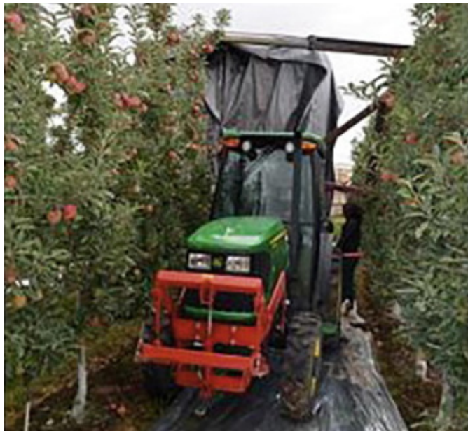
FIGURE 3: OVER-THE-ROW (OTR) SENSOR PLATFORM WITH A TUNNEL STRUCTURE. 5
