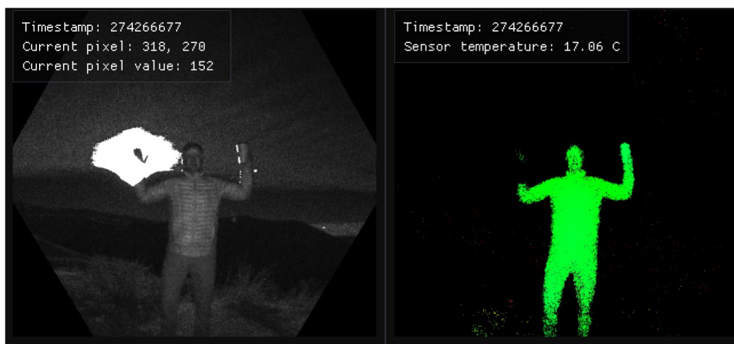
FIGURE 1: EXAMPLE OF AN ACTIVE STEREO DEPTH SENSOR FAILING IN SUNLIGHT
