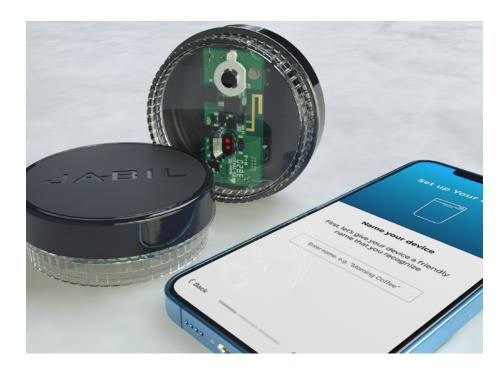
Connected Packaging provides an exciting solution to many of the challenges that the world's largest CPGs currently face. Jabil's connected packaging solution combines three key elements: the durable device, the consumable package and the companion app.
